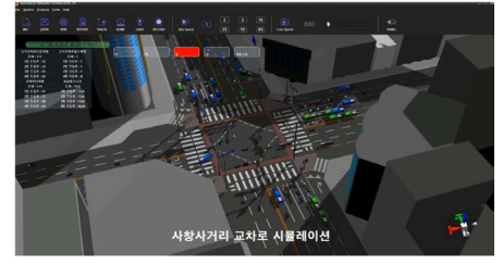
Smart city traffic simulation based on traffic light control
